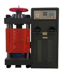
**Hydraulic system:** The hydraulic oil in the oil tank enter the oil circuit through the motor drives the high-pressure pump, flows through the return oil valve, and into the oil cylinder. The force measuring instrument collects and analyzes the data through the sensor, showing the constant force value. The operator through the delivery valve to adjust the flow and control the test force rate.
